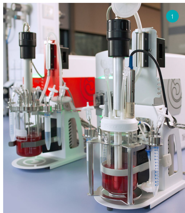
Figure 1 | Single-use and autoclavable glass mini-bioreactor (Applikon Biotechnology).
